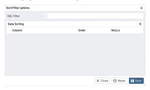
• Use *SQL Filter* to provide SQL filtering criteria. These will be added to the "WHERE" clause of the query used to retrieve the data. For example, you might enter:
