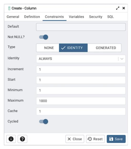
Use the following fields to create *IDENTITY* column. Identity columns are applicable for PG/EPAS version 10 and above.
