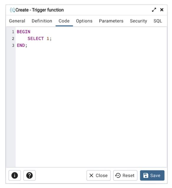
• Use the *Code* field to write the code that will execute when the trigger function is called.
