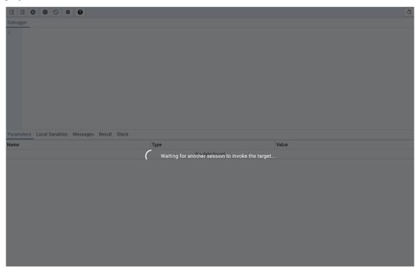
When another session invokes the target, the debugger will display the code, allowing you to add break points, or step through line-by-line. The other session is suspended until the debugging completes; then control is returned to the session.
