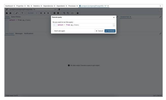
The message returned by the server when a command executes is displayed on the *Messages* tab. If the command is successful, the *Messages* tab displays execution details.
