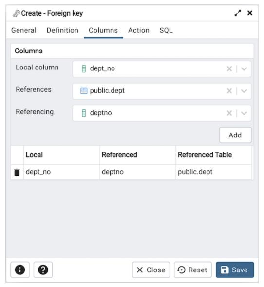
Use the fields in the *Columns* tab to specify one or more reference column(s). A Foreign Key constraint requires that one or more columns of a table must only contain values that match values in the referenced column(s) of a row of a referenced table:
