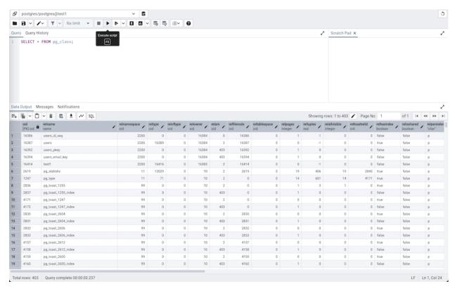
You can also execute a query based on cursor position. Query tool will detect a query and underline it when cursor position changes. Now, to execute the current underlined query, hit the *Execute query* button on the toolbar. If a section is highlighted then it will behave like normal execute.
