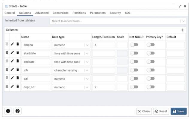
Use the drop-down listbox next to *Inherited from table(s)* to specify any parent table(s); the table will inherit columns from the selected parent table(s). Click inside the *Inherited from table(s)* field to select a table name from a drop-down list. Repeat to add any other parent tables. Delete a selected table by clicking the *x* to the left of the parent name. Note that inherited column names and datatypes are not editable in the current dialog; they must be modified at the parent level.
