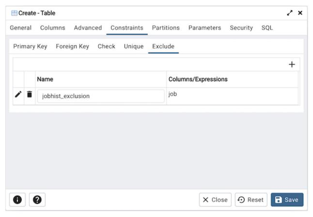
To add an exclusion constraint, select the *Exclude* tab on the panel, and click the *Add* icon (+). To define the constraint, click the *Edit* icon to the left of the *Trash* icon. A dialog similar to the *Exclusion constraint* dialog (accessed by right clicking on *Constraints* in the *pgAdmin* tree control) opens.
