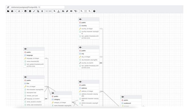
You can open multiple copies of the ERD tool in individual tabs simultaneously. You can also generate an ERD from a database, schema or a table.
