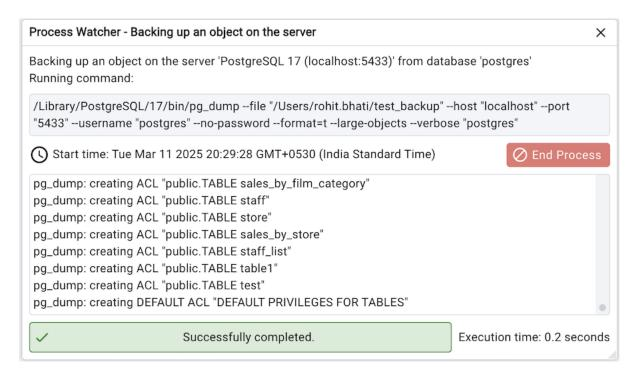
The Process Watcher logs all the activity associated with the process/task and provides additional information for troubleshooting Use the **End Process** button to end the process.
